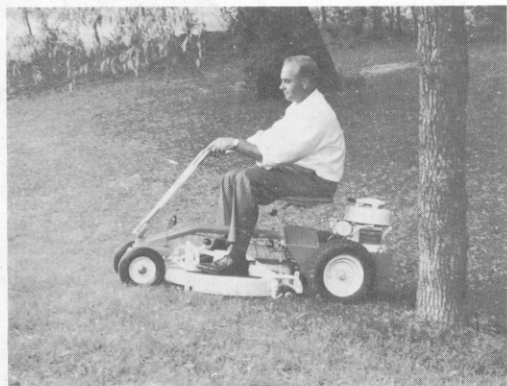
ARIENS EMPEROR riding mower. Available with Flex-N-Float 26" or 32" rotary or 30" reel mower; Insta-hitch attachments. Electric or recoil starting 5½ h.p. engine.
