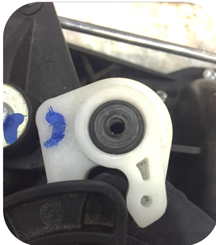
Reference photo VA11: White lever correct position
