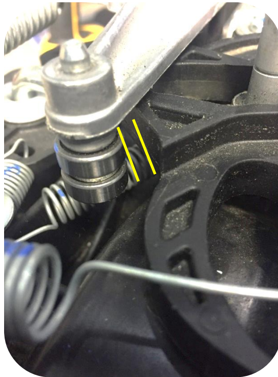
Reference photo VA12: Control cam 5mm gap
