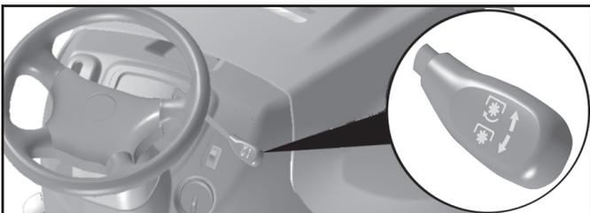
(☒) ATTACHMENT CLUTCH SWITCH “DISENGAGED”
