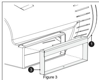
Position mounting bracket assembly on top of frame and secure top edge with two 3/8" x 1" hex bolts (item 4), two 13/32" x 13/16" flat washers (item 5) and two 3/8" center locking flange nuts (item 6). See Figure 4.
