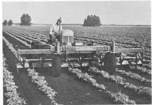
ARIENS TILLIVATOR. Tractor mounted, custom-built tillers for large scale vegetable growers.
