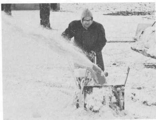
ARIENS SNO-THRO Self propelled, 2 stage, heavy duty, 3½ h.p. or 5½ h.p. rotary snow thrower. 180° swiveling SNO-CHUTE with hand crank directional control.
