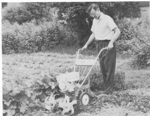
ARIENS SUPER JET rotary tiller with TURBO TINES. 24" tilling width. Choice of 4 famous make engines—3 h.p. to 4½ h.p. with tine reverse drive.
