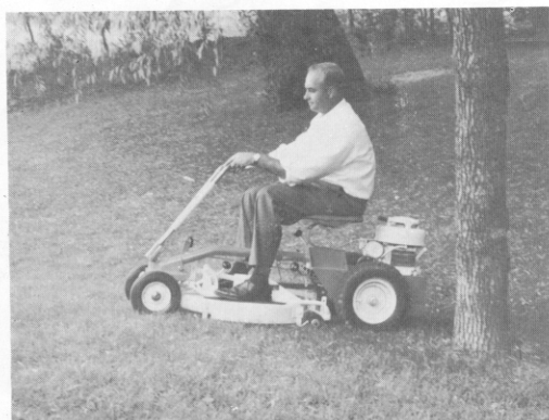
ARIENS EMPEROR riding mower. Available with Flex-N-Floot 26" or 34" rotary or 26" reel mower; Insta-hitch attachments. Electric or recoil starting 5½ h.p. engine.
