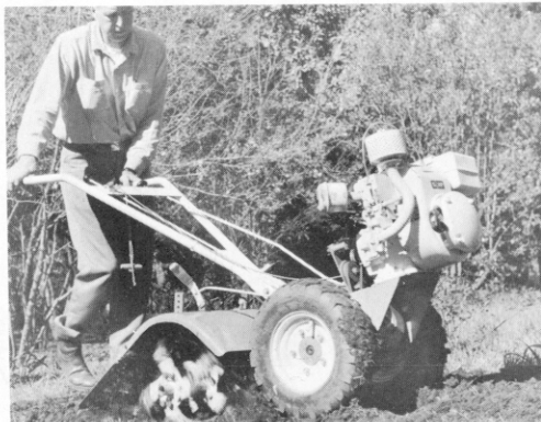
ARIENS ROCKET rotary tiller with TURBO TINES and friction-drive Tine Reverse. 20" tilling width. 5½ h.p. Lauson engine. For commercial, professional and home gardener use.
