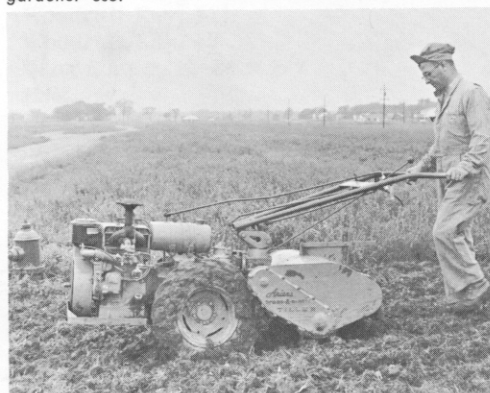
ARIENS TRANS-A-MATIC for heavy duty commercial tilling. Choice 9.0 h.p. or 16.5 h.p. Wisconsin engine; 20" or 28" tilling widths. Non-slip differential.
