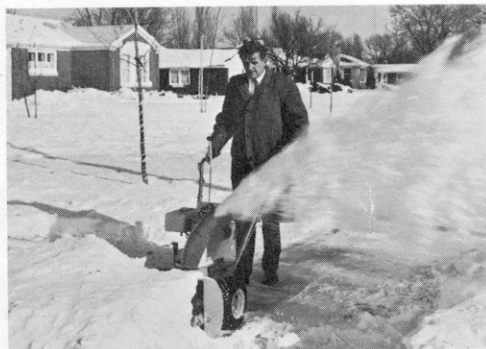
ARIENS SNO-THRO Self propelled, 2 stage, heavy duty, 3½ or 6 h.p. rotary snow thrower. 180° swiveling SNO-CHUTE with hand crank directional control.
