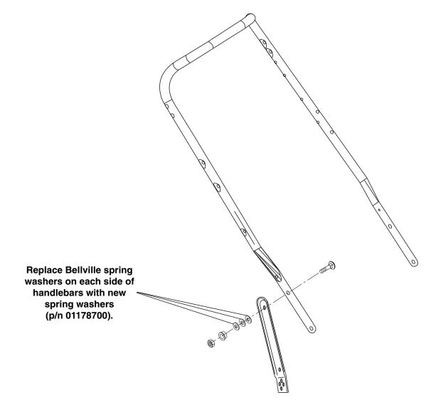
**Please Note:** Part number 01178700 is not being changed in our parts system. Replace faulty parts with new parts of the same part number.
