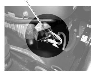
If the ground wires were connected to the voltage regulator, connect the solenoid and battery ground wires here instead. **NOTE:** Make sure the ground wires get good metal to metal contact with the seat spring plate. You may need to scrape away some paint to make a good ground contact.
