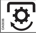
Engages and disengages attachment. Pull switch to engage; push switch to disengage.
