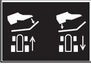
Press front of pedal down to move unit forward.
